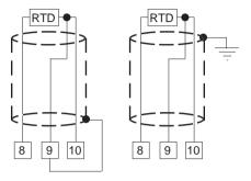
Fig. 5 RTD INPUT WIRING
